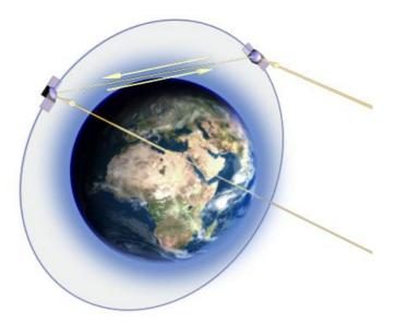
Through sensing of Earth atmosphere is implemented by light beam radiated from the board of one satellite through atmosphere mass towards to another satellite.
